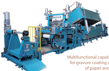
Roll-to-roll coating and lamination line at Fraunhofer IVV
