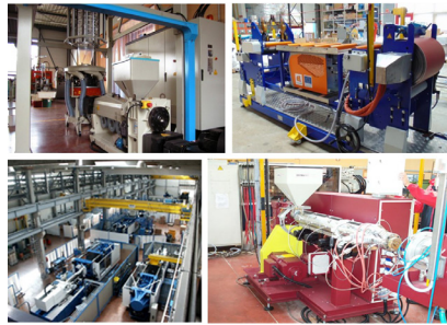
Examples of converting steps: (top): blown film extrusion, film take-off station, (bottom): injection molding facility, tube and profile extrusion machine (at IPC)
